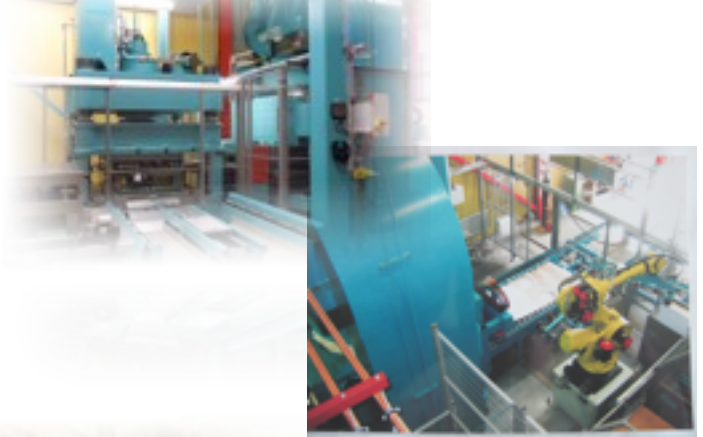
12500T PHE' s Plates Production Line in Sweden
