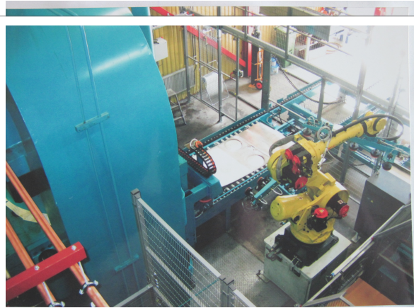
12500T PHE' s Plates Production Line in Sweden
